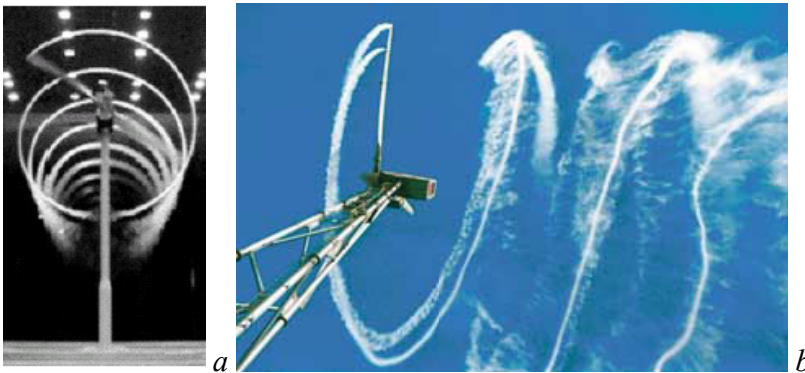
Fig. 1. Visualisations of far wake: (a) stable regime [4] and (b) unstable one with the wake decay (data by RISO, Denmark).
