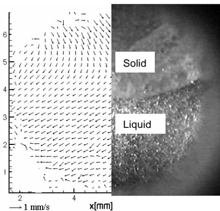
Figure 3: Convective processes during melting of Ice I
