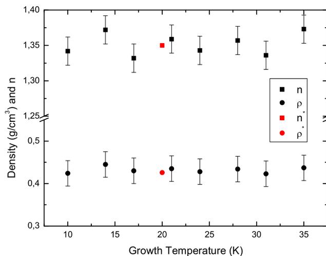
Figure 2. Density and real part of the index of refraction for methane as a function of the growth temperature
