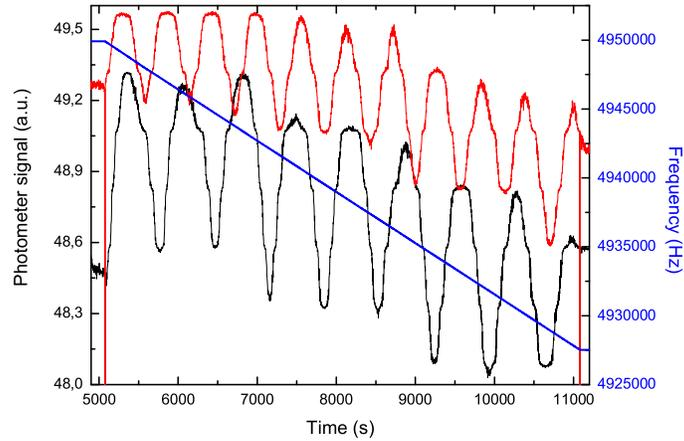
Figure 1. Ice film deposit. Blue line, velocity of deposition. Red interference pattern incidence 27 degrees. Black interference pattern incidence 63 degrees.
