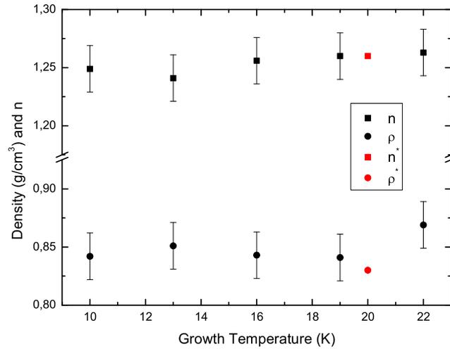
Figure 3. Density and real part of the index of refraction for nitrogen as a function of the growth temperature
