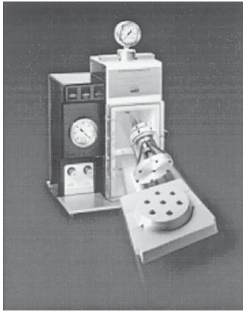
Fig. 2. Biolistic PDS/1000He with sevenfold pressure distribute.
