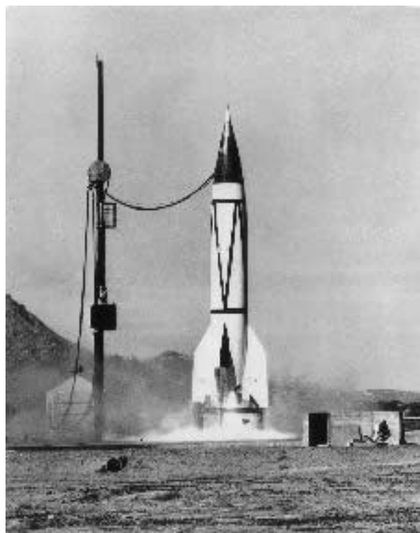
Figure 2 A V-2 rocket just prior to launch at the White Sands Proving Ground in New Mexico. About 45 feet tall and 5 feet in diameter it was fueled by 10 tons of alcohol and liquid oxygen. The rocket is shown connected by an umbilical cable to the firing line. To service the rocket and its payload a portable ladder was brought up. Only later was a gantry provided from which each level of the rocket could be reached comfortably. A successful flight could reach 170 \text{ km} and last for 450 \text{ sec} . (NRL.)
