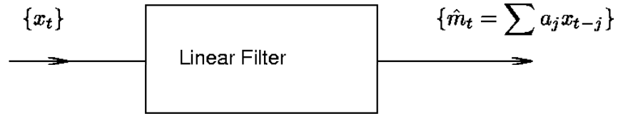
Figure 1-20 Smoothing with a low-pass linear filter.
