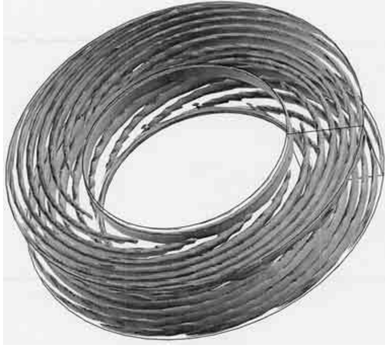
FIGURE 7.4. Instantaneous iso-surface of the axial velocity component ( w = -3.5 \times 10^{-4} ) of the time-periodic three-dimensional flow for C_w = 530 , E = 2.24 \times 10^{-3} , L = 3.37 and R_m = 5 .
