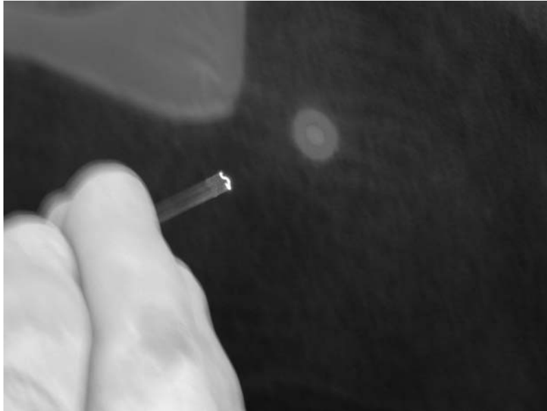
Figure 10.24. A sharp, round laser spot indicating good focus. (See color insert)
