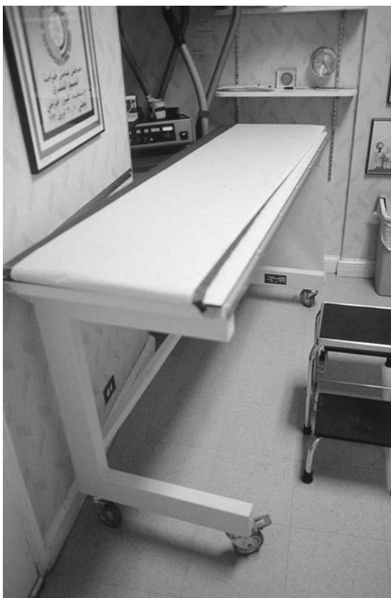
Figure 10.1. Radiolucent table on casters allows maximal movement of the patient and permits millimeter-by-millimeter adjustment in relation to the x-ray tube for optimal imaging.
