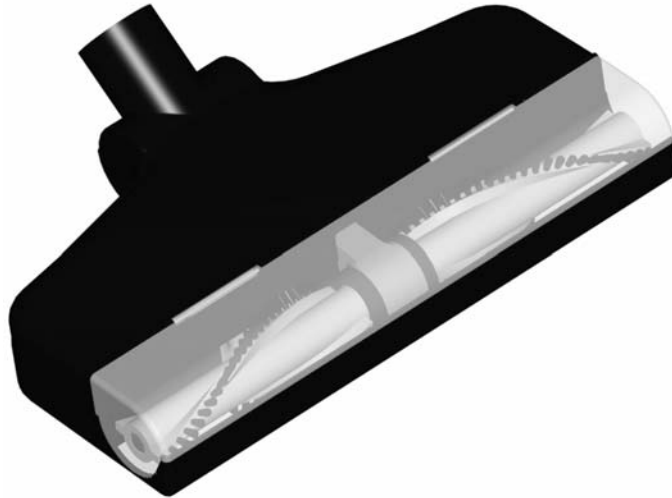
Fig. 2.20. Brush cleaner head with transparent cover
