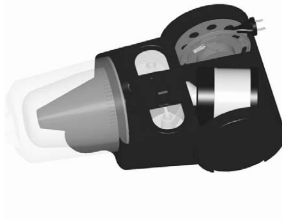
Fig. 2.23. CAD prototype design of the vacuum cleaner
