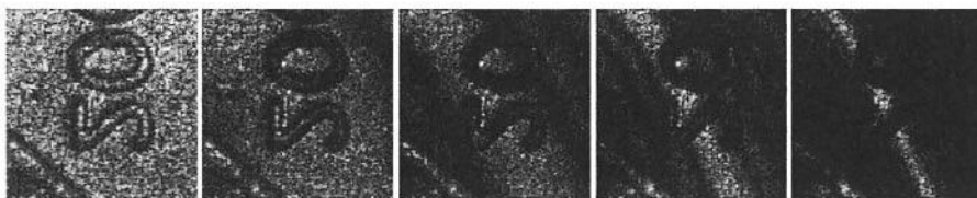
Figure 2-12. Build up of axial resolution by superposition of holographic images of a penny using a range of wavelengths with N = 1, 2, 4, 8 , and 20 .
