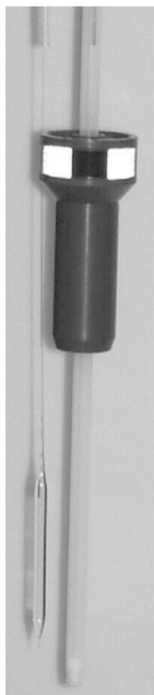
Fig. 2. A pressure-resisting quartz cell and the protecting Teflon capsule used for the on-line cell high-pressure nuclear magnetic resonance system.
