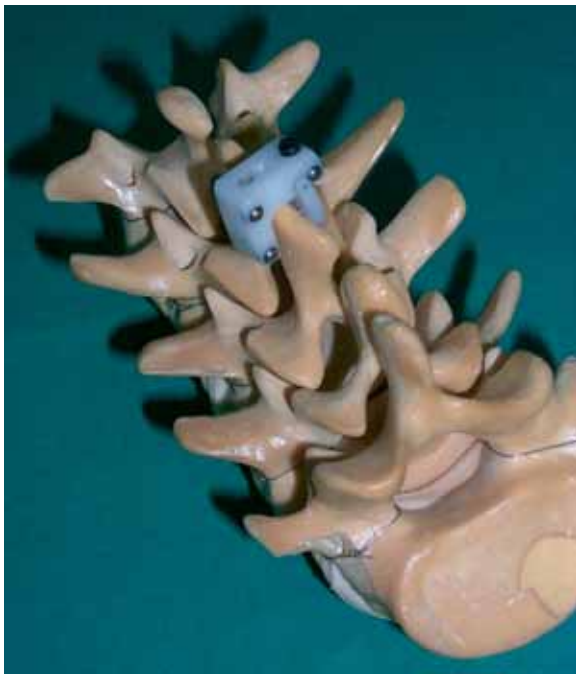
Fig. 6.4. This base part of a prototype dynamic reference base is mounted to the spinous process prior to CT data acquisition. The three high-precision titanium spheres help registering the device with the image data in an automatic way
