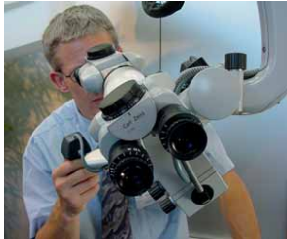
Fig. 3.2. Adjustment of microscope position, focus, magnification, and working distance with the handpiece
