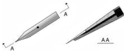
fig. 2.5. Essential construction of a pen
