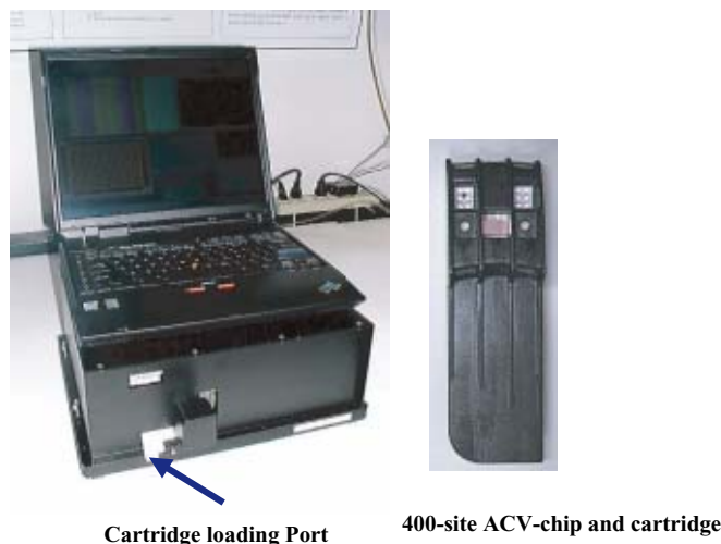
FIGURE 1.12. Photograph of the electronic microarray system with the laptop used to operate the instrument and perform data storage and processing. The arrow indicates a port for the 400-site cartridge introduction.
