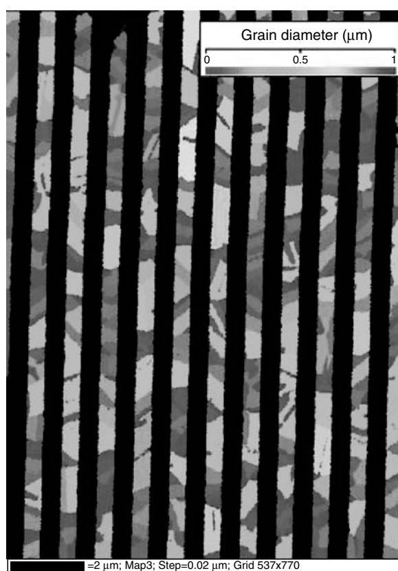
FIGURE 2.34. Grain size (equivalent-circle diameter) map, with all \Sigma 3 twins as grain-delimiting boundaries. Scale bar = 2 μm (see color insert).
