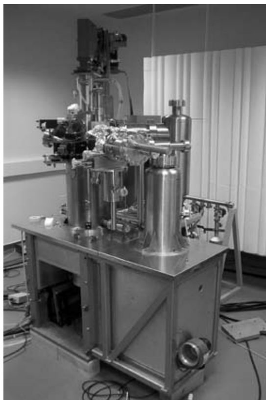
FIGURE 2-2. A photograph of a dedicated STEM instrument (VG Microscopes HB501). The gun is below the table level, with most of the electron optics above the table. At the top of the column can be seen a magnetic prism spectrometer for electron energy-loss spectroscopy.
