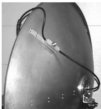
Figure 3. Splitter with feed cables mounted on back side of IRA-6.
