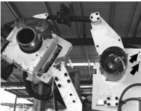
Figure 2.44 Airknife support head and its various adjustments. The arrows show where the flange bolts sheared off
