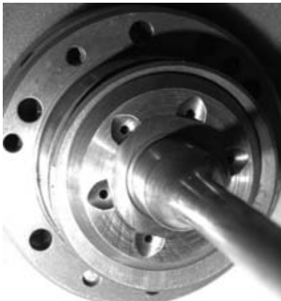
Figure 2.53 Nominally worn thrust face of high-speed shaft replaced in overhaul
