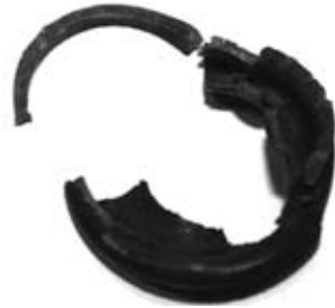
Figure 2.74 Sealing boot parts recovered from the failed joint
