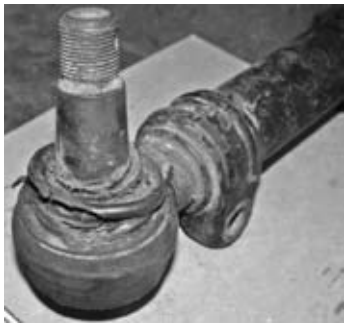
Figure 2.58 Original design of track rod (worn sample from Fillyary)
