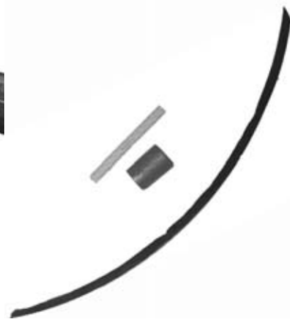
Figure 2.13 Part of the bearing broken away during the accident, with a roller and a 300 mm ruler to indicate scale
