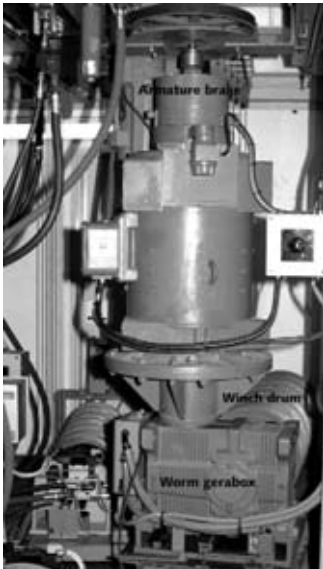
Figure 2.3 A winch motor and gearing system. The motor drive is attached to a worm gearbox
