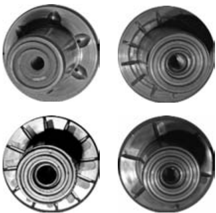
Figure 2.54 Original thrust face compared to various alternatives tried by Electra
