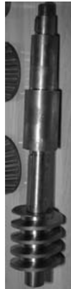
Figure 2.5 Typical motor shaft and worm screw
