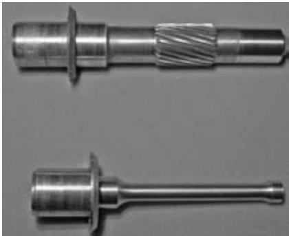
Figure 2.50 High-speed pinion assembly and separated inner shaft
