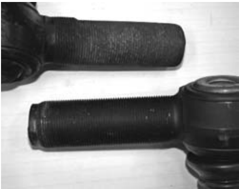
Figure 2.61 Worn knuckle (top) and new knuckle (bottom)
