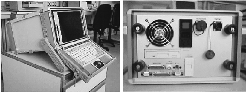
Figure 2.1. PQ meter open platform designed at the Department of Electrical Engineering, University of Cantabria
