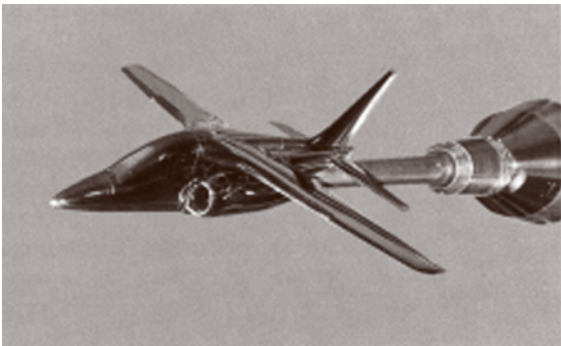
Fig. 8.13 Tail sting through engine nozzle
