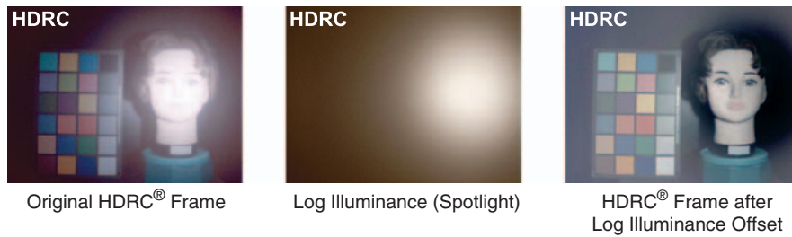
Fig. 1.9. One frame from a video sequence of a moving model with spot illumination recorded with an HDRC camera. On the left: The raw frame. In the middle: The log profile of the illumination recorded and stored after the installation of the camera. On the right: The illumination profile added as an offset in real time to the raw frame. Frame rate: 30 \text{ frames s}^{-1}
