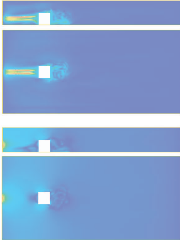
Fig. 1.4. From Chapter 15: Surface mounted cube: dual velocity |\varphi_h| (upper), and dual pressure |\iota_h| (middle), in the x_1x_2 -plane at x_3 = 3.5H and in the x_1x_3 -plane at x_2 = 0.5H .
