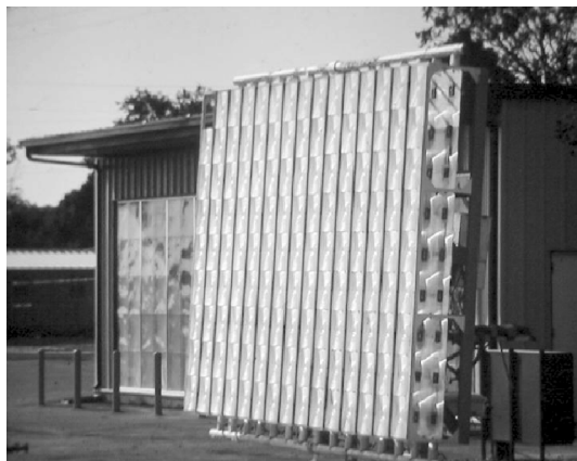
Fig. 1.2. The SANDIA-II array, the first modern PV concentrator made at Sandia National Laboratories, Albuquerque, New Mexico, in 1977. It consists of 5-cm-diameter Si cells operating on two axes under cast acrylic Fresnel lenses at 32 suns, with passive cooling
