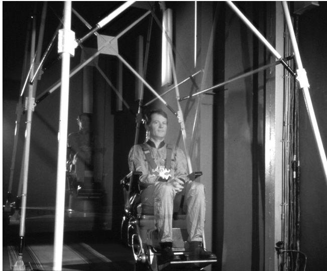
Figure 2-01. The Khilov's swing test was used in Star City (near Moscow, Russia) for selection and training of cosmonauts. Here, a French cosmonaut sat in a chair suspended from the top of a four-post structure. The fore-aft translation of the swing generated linear accelerations that stimulated the otolith organs of his vestibular system. Photo courtesy of CNES.
