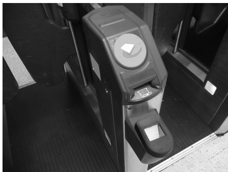
Fig. 2.3. An RFID ticket validator at the gates of the London Underground network.
