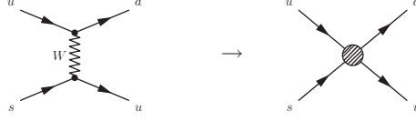
Fig. 4. At low energies the single W boson exchange reduces to a four-quark contact interaction.
