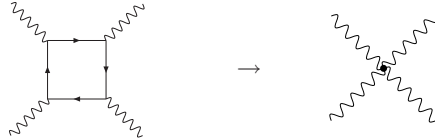
Fig. 3. The one-loop diagram of QED is replaced in the effective theory by 4-photon contact interactions.
