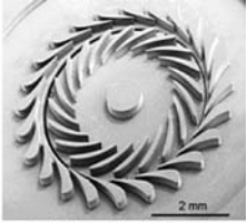
Microturbine bladed rotor and nozzle guide vanes on the stator (Spearing and Chen, 2001)
