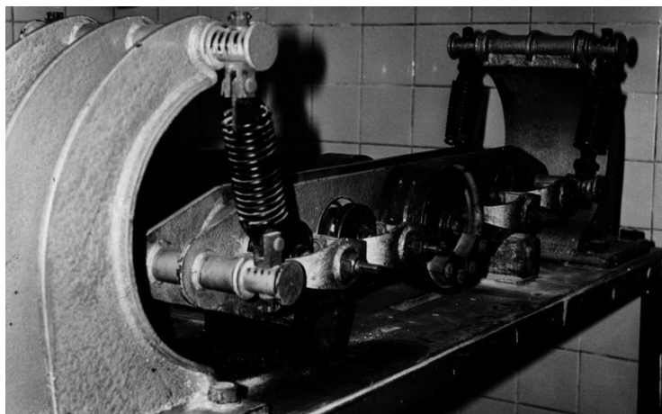
Fig. 2.6 Laboratory vibration mill
