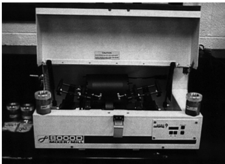
Fig. 2.12 Laboratory mixer mill Spex 8000 (CertiPrep, USA) [ http://www.utk.edu ]
