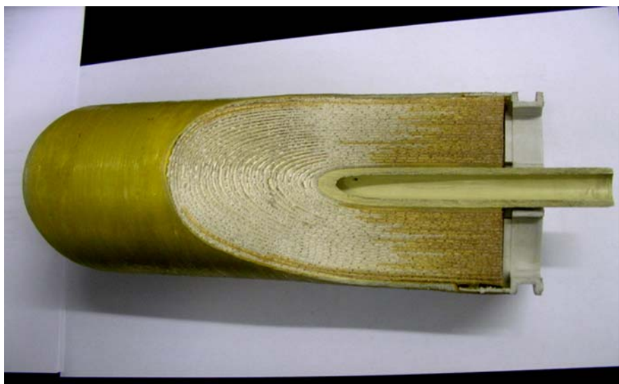
Fig. 5 Spiral-wound membrane part
