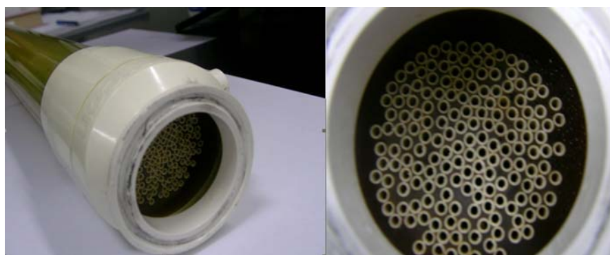
Fig. 3 Hollow-fiber (HF) membrane module
