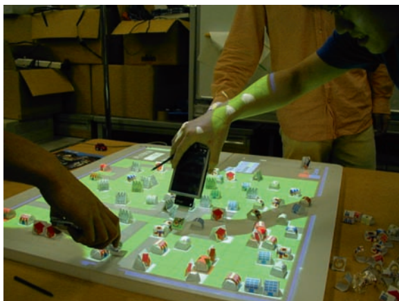
Fig. 11 By bringing a PDA near an area of interest in the shared workspace, the corresponding area appears on the personal workspace
