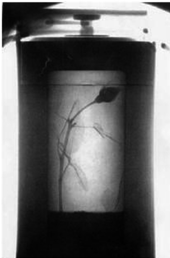
Fig. 3 Neutron radiograph of a rose in a lead flask [5]
