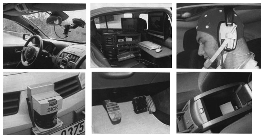
Fig. 3.3 Vehicle sensors: cameras, navigator area and instruments bench, laser range finder, 3D accelerator, brake pressure sensor, microphone, and EEG cap (from top left clockwise.)
