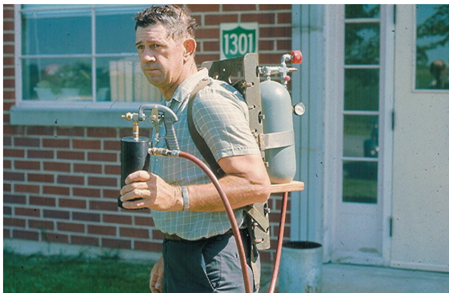
Fig. 2.3 A 1970 photograph of the hand applicator used in the initial defoliant screening tests at Fort Detrick. The sprayer was a specially calibrated unit capable of delivery less than 0.1 kg/ha of candidate defoliants (photograph courtesy of A. Young)
