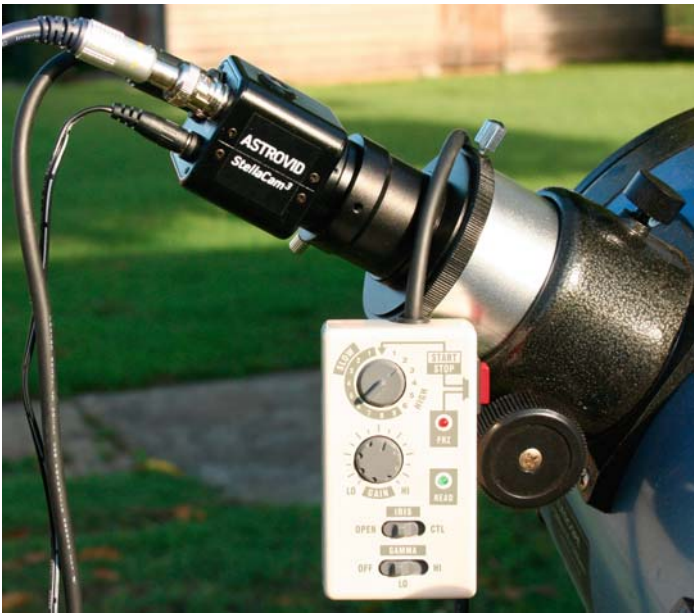
Fig. 2.5. StellaCam 3 fitted to a Newtonian telescope. Courtesy of Phillip Hinkler.
