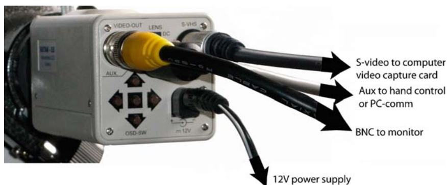
Fig. 2.13. Back panel connections of the GSTAR-EX camera.
