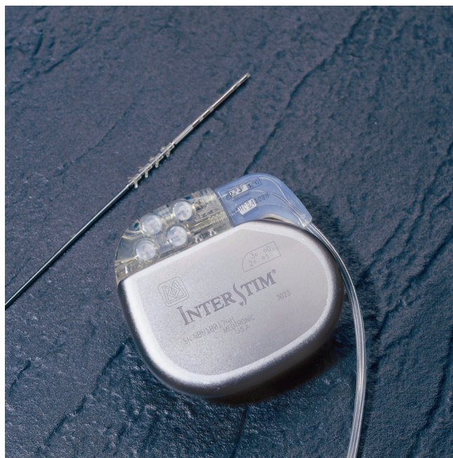
FIGURE 14.6. SNS InterStim device. (With permission of Medtronic, Inc., © 2008.)
