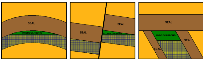
Fig. 2.2 Structural traps: anticlinal trap (left) and fault trap (middle). Stratigraphic trap (right): tilted layers of varying permeability
