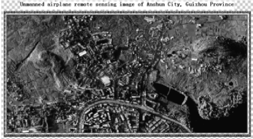
Fig. 2.17 Image spliced by images photographed at an altitude of 1km
