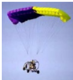
Fig. 2.3 An unmanned powered paraglider (Thamm and Judex 2006)
