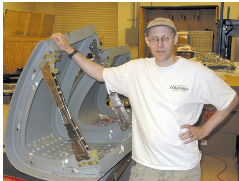
Fig. 2.14 RCC Leading Edge with T-Seal.
