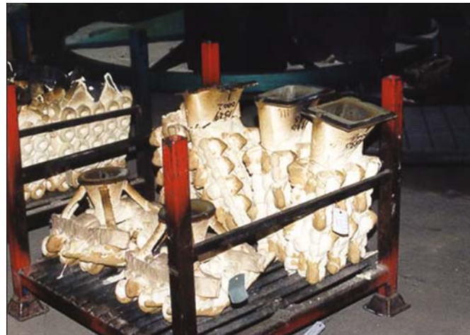
FIG. 2.24. Molds on foundry cooling rack after casting.
