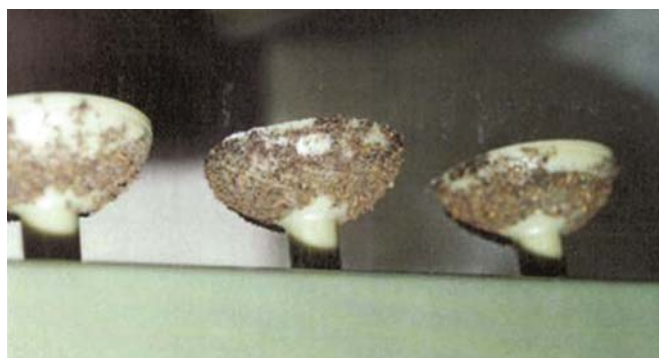
FIG. 2.36. Wax pattern covered in tea leaves on a wax runner.
