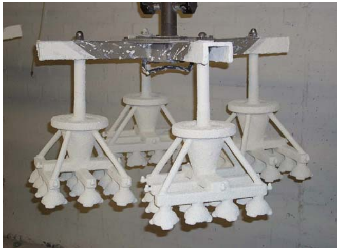
FIG. 2.19. Wax assemblies supported by a robotic arm for shelling.
