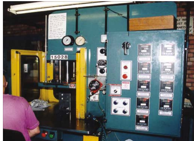
FIG. 2.18. Wax injection machine, or press, injecting wax into a wax pattern tool.
