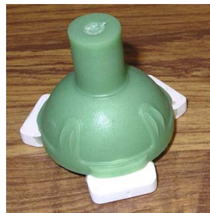
FIG. 2.16. A wax pattern of an acetabular cup showing the gate on the convex surface and three ceramic core prints.
