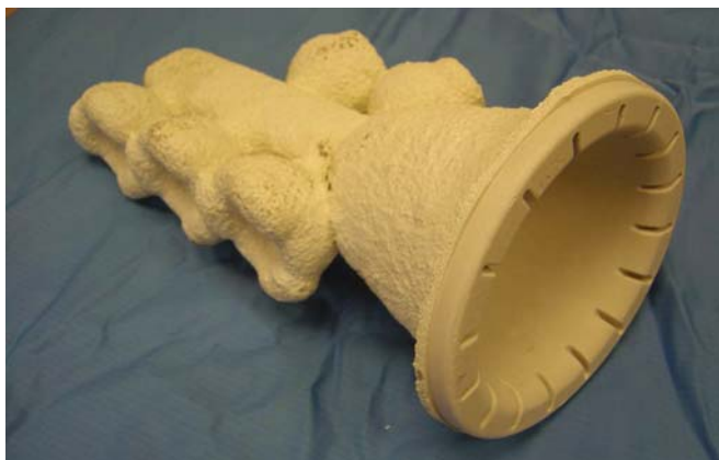
FIG. 2.20. Ceramic shell after dewaxing and flash-firing.
