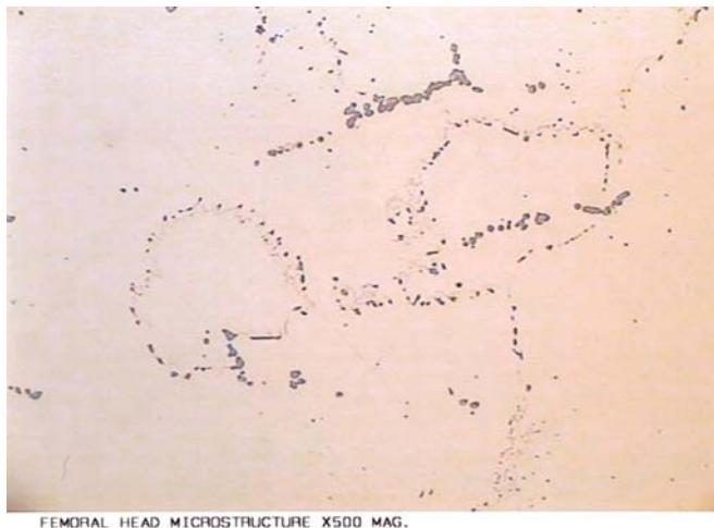
FIG. 2.33. CoCr cast alloy after sintering, HIP and SHT.
