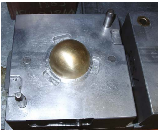
FIG. 2.15. View inside a wax pattern tool cavity of an acetabular cup with three ceramic core print locations.
