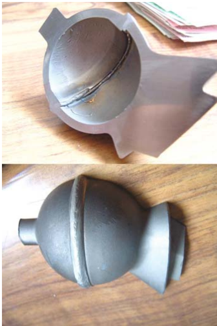
FIG. 2.5. Cross section of a two-piece assembly of the hollow femoral device in an electron beam welded condition.
