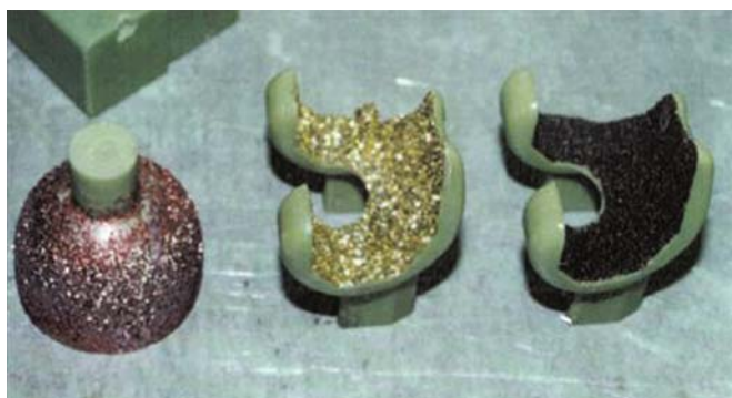
FIG. 2.35. Wax pattern covered in decorative glitter.
