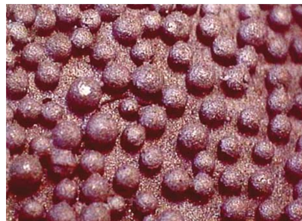
FIG. 2.42. (A) BHR cup with Porocast surface; (B) high magnification of beaded surface.
