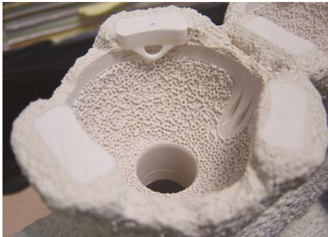
FIG. 2.38. A section of a shell showing the detail of the Porocast structure.
