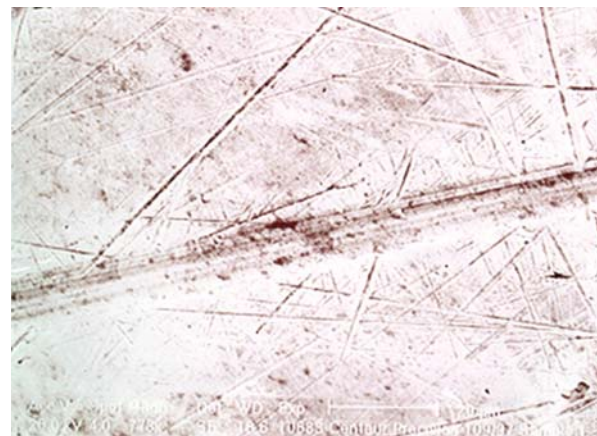
FIG. 2.8. Scratches on bearing surface.
