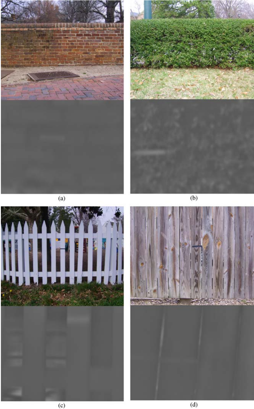
Fig. 2.13 Visible and thermal images of extended objects from the training data set. (a) brick wall, (b) hedges, (c) wood picket fence, and (d) wood wall.
