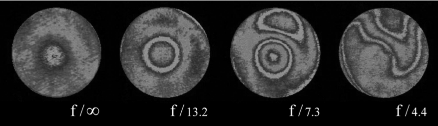
Fig. 2.14 Optical tests of a Type 2 VCM with respect to concave calibers. Zoom range f/\infty - f/4.5 . He-Ne patterns for full aperture 2a = 16\text{ mm} . The central force is varied from 0 to 5.85\text{ daN} (LOOM)
