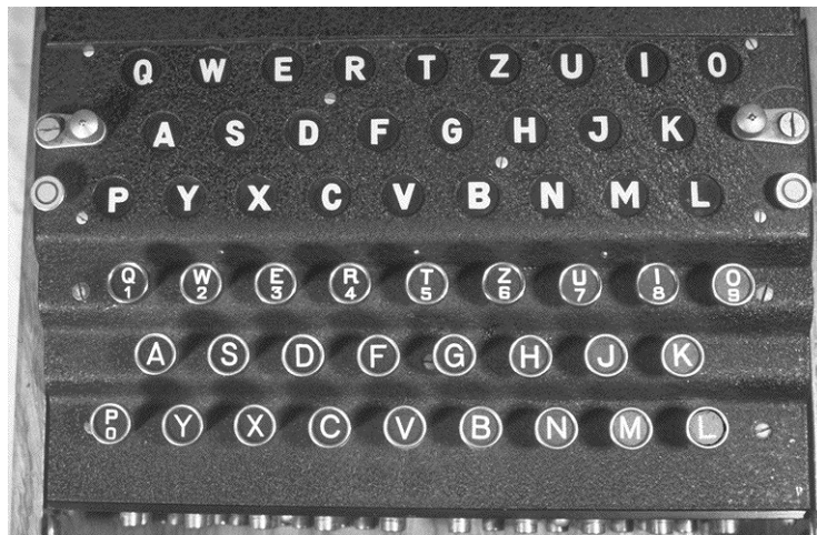
Fig. 7.1. Enigma's keyboard and display
