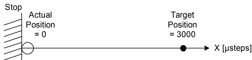
Figure 23: Positioning Example: Situation after reference search
