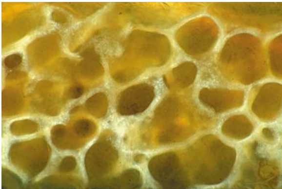
Fig. 2.7. Surface of a trimmed plastic block showing a fairly uniform trabecular network
