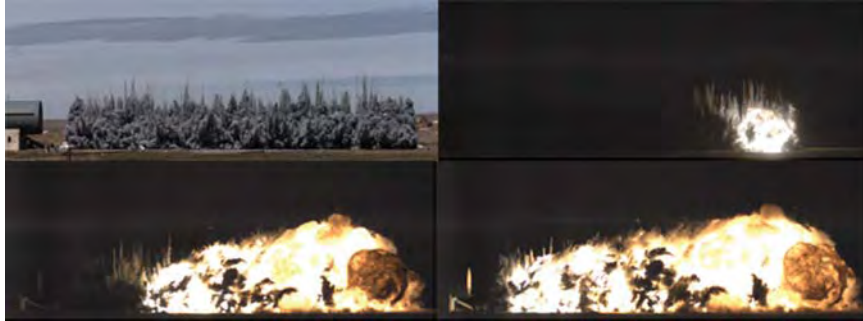
Fig. 2.22. DDT in an unconfined 3\text{ m} \times 3\text{ m} \times 18\text{ m} flaked aluminum–air cloud. Top left: Aluminum suspension. Top right: 8 kg C4 explosive initiation. Bottom left and bottom right: Detonation propagation [22]
