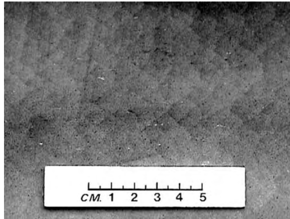
Fig. 2.39. Cellular detonation structure for the type-I weak hybrid detonation in a mixture of \phi = 0.8 C_2H_2 -air and 500\text{ g m}^{-3} , 10\text{-}\mu\text{m} (H-10) aluminum particles [32]
