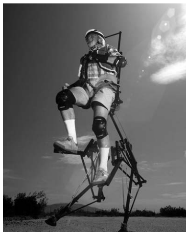
Fig. 2.18 Exoskeleton supporting walking motion [Photo courtesy of B. SMALE]
