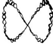
Fig. 1.4. Observed trajectory of a microparticle in a Paul-type trap [6]
