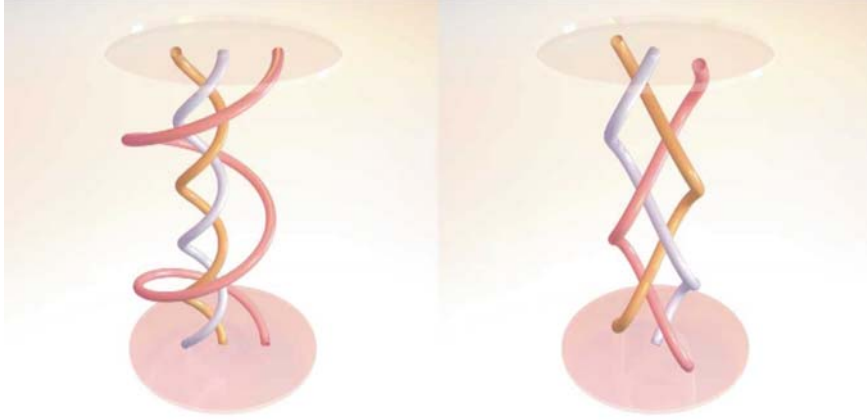
Fig. 10 Two braids. The left braid only exhibits ordinary (first order) winding. The right figure shows a pigtail braid with second order winding.
