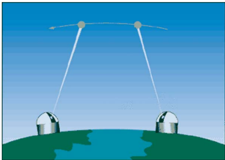
Fig. 2.7. Principle of satellite laser ranging.
